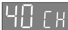
During Auto Channel Set The channel numbers are displayed as they are scanned and set.
